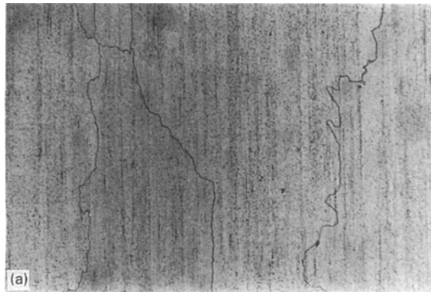
Figure 3 Microstructure of MA760 obtained after zone annealing normal to the extrusion direction (vertical). (a) 0.8 \text{ mm min}^{-1} ; the sample went through the zone-annealing furnace without interruption. (b) 5.6 \text{ mm min}^{-1} . The sample travel direction is from left to right of the micrographs. The darker etching region in (b) is unrecrystallized.
